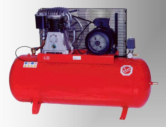
Oil-free, dual cylinders with twin stage compression engine, 4 HP (3 kW) high performances compressor, suited to supply a battery of several standards and/or high pressure SM-8850 WRT machines coupled to pressure boosters.
